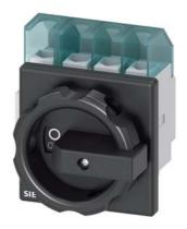
SENTRON, Switch disconnector 3LD, main switch, 4-pole, lu: 25 A, Operating power / at AC-23 A at 400 V: 9.5 kW, front-mounted, rotary operating mechanism, black, 4-hole mounting of the handle
