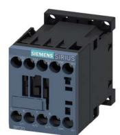
power contactor, AC-3e/AC-3, 7 A, 3 kW / 400 V, 3-pole, 220 V DC, auxiliary contacts: 1 NC, screw terminal
