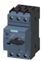
Circuit breaker size S00 for motor protection, CLASS 10 A-release 4.5...6.3 A N-release 82 A screw terminal Standard switching capacity
