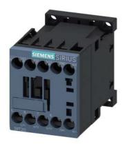
power contactor, AC-3e/AC-3, 7 A, 3 kW / 400 V, 3-pole, 24 V DC, 0.7-1.25  $^{\star}$  Us, with integrated suppressor diode, auxiliary contacts: 1 NC, screw terminal, suitable for PLC outputs, not expandable with auxiliary switch
