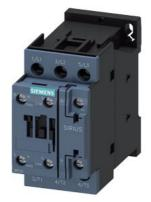
power contactor, AC-3e/AC-3, 17 A, 7.5 kW / 400 V, 3-pole, 24 V AC, 50/60 Hz, auxiliary contacts: 1 NO + 1 NC, screw terminal
