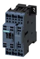
power contactor, AC-3e/AC-3, 32 A, 15 kW / 400 V, 3-pole, 24 V DC, auxiliary contacts: 1 NO + 1 NC, spring-loaded terminal
