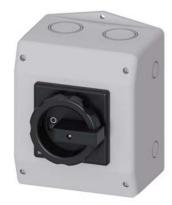
SENTRON, Switch disconnector 3LD, main switch, 6-pole, lu: 25 A, Operating power / at AC-23 A at 400 V: 9.5 kW, molded-plastic encapsulation for metric cable gland, rotary operating mechanism, black
