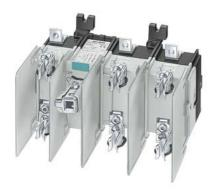
Switch disconnector with fuse in new design Iu=125 A, Ue=690 V, 3-pole for LV HRC fuse Sz. 00 basic version without 8UC6 handle and shaft
