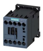
power contactor, AC-3e/AC-3, 9 A, 4 kW / 400 V, 3-pole, 230 V AC, 50/60 Hz, auxiliary contacts: 1 NO, screw terminal, upright mounting position
