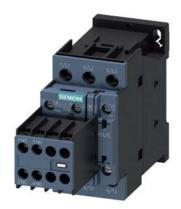
power contactor, AC-3e/AC-3, 25 A, 11 kW / 400 V, 3-pole, 24 V AC, 50 Hz, auxiliary contacts: 2 NO + 2 NC, screw terminal, removable auxiliary switch
