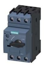
Special type Circuit breaker size S00 for motor protection, CLASS 10 Arelease 2.8...4 A N release 52 A screw terminal Standard switching capacity Ambient temperature -50  $^{\circ}\text{C}$  500 switching cycles
