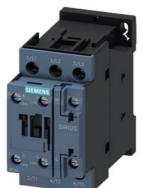
power contactor, AC-3e/AC-3, 12 A, 5.5 kW / 400 V, 3-pole, 24 V AC, 50 Hz, auxiliary contacts: 1 NO + 1 NC, screw terminal
