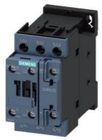
power contactor, AC-3e/AC-3, 12 A, 5.5 kW / 400 V, 3-pole, 110 V AC, 50 Hz, auxiliary contacts: 1 NO + 1 NC, screw terminal
