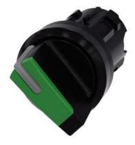
Selector switch, illuminable, 22 mm, round, plastic, green, selector switch, short, 2 switch positions O-I, latching, actuating angle 90°, 10:30h/13:30h
