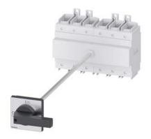
SENTRON, Switch disconnector 3LD, main switch, 6-pole, lu: 160 A, Operating power / at AC-23 A at 400 V: 75 kW, floor mounting with door coupling, knob-operated mechanism, black, 4-hole mounting of the handle
