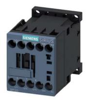
power contactor, AC-3e/AC-3, 7 A, 3 kW / 400 V, 3-pole, 24 V DC, 0.7-1.25\* Us, auxiliary contacts: 1 NC, screw terminal, suitable for PLC outputs, not expandable with auxiliary switch
