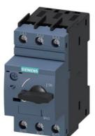
Special type Circuit breaker size S0 for motor protection, CLASS 10 A-release 34...40 A N-release 480 A screw terminal Standard switching capacity Ambient temperature -50 °C 500 switching cycles
