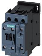
power contactor, AC-3e/AC-3, 32 A, 15 kW / 400 V, 3-pole, 110 V AC, 50/60 Hz, auxiliary contacts: 1 NO + 1 NC, screw terminal
