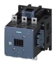
power contactor, AC-3e/AC-3 400 A, 200 kW / 400 V AC (50-60 Hz) / DC Uc: 110-127 V 3-pole, auxiliary contacts 2 NO + 2 NC drive: conventional main circuit: busbar control and auxiliary circuit: screw terminal
