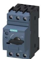
Special type Circuit breaker size S00 for motor protection, CLASS 10 A-release 5.5...8 A N-release 104 A screw terminal Standard switching capacity Ambient temperature -50  $^\circ$ C 500 switching cycles
