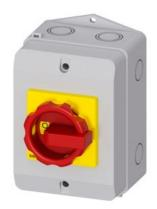
SENTRON, Switch disconnector 3LD, emergency switching-off switch, 4-pole, 16 A, operating power at AC-23 A at 400 V: 7.5 kW, molded-plastic encapsulation for metric cable gland, rotary operating mechanism, red/yellow
