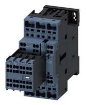
power contactor, AC-3e/AC-3, 25 A, 11 kW / 400 V, 3-pole, 24 V AC, 50 Hz, auxiliary contacts: 2 NO + 2 NC, spring-loaded terminal, removable auxiliary switch
