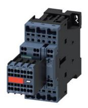
power contactor, AC-3e/AC-3, 25 A, 11 kW / 400 V, 3-pole, 24 V DC, with plugged-in diode combination, auxiliary contacts: 2 NO + 2 NC, spring-loaded terminal, captive auxiliary switch
