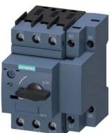
Circuit breaker size S00 for motor protection, CLASS 10 with overload relay function A-release 2.2...3.2 A N release 42 A screw terminal Standard switching capacity
