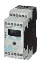
temperature monitoring relay Thermocouple J, T, E, K, N 2 threshold values digitally adjustable -99 °C to 999 °C 24 - 240 V AC/DC 2 x 1 CO + 1 NO, width 45 mm screw terminal !!!phased-out product!!! the preferred successor is 3RS2600-2BW30
