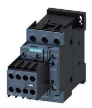
power contactor, AC-3e/AC-3, 17 A, 7.5 kW / 400 V, 3-pole, 110 V AC, 50 Hz, auxiliary contacts: 2 NO + 2 NC, screw terminal, removable auxiliary switch
