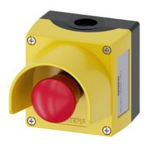
Enclosure for command devices, 22 mm, round, Enclosure material plastic, Enclosure top part yellow, 1 control point plastic, with protective collar, A=EMERGENCY STOP mushroom pushbutton red, 40 mm, rotate-to-unlatch, 1 NC, screw terminal, floor mounting, 1xM20 each on top and bottom
