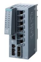
SCALANCE XC206-2SFP manageable Layer 2 IE switch; IEC 62443-4-2 certified; 6x 10/100 MBit/s RJ45 ports; 2x 100/1000 Mbit/s SFP; 1x console port; diagnostics LED; redundant power supply; temperature range -40 °C to +70 °C; assembly: DIN rail/S7 mounting rail/wall Office redundancy functions features (RSTP, VLAN,...); PROFINET IO device; Ethernet/IP-compliant; C-plug slot;
