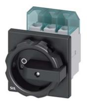
SENTRON, Switch disconnector 3LD, main switch, 3-pole, lu: 25 A, Operating power / at AC-23 A at 400 V: 9.5 kW, front-mounted, rotary operating mechanism, black, 4-hole mounting of the handle
