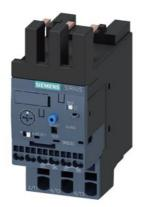
Overload relay 10...40 A Electronic For motor protection Size S0, Class 10E Contactor mounting Main circuit: Spring-type terminal Auxiliary circuit: Spring-type terminal Manual-Automatic-Reset
