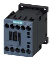
power contactor, AC-3e/AC-3, 9 A, 4 kW / 400 V, 3-pole, 24 V DC, 0.7-1.25\* Us, with integrated diode, auxiliary contacts: 1 NO, screw terminal, suitable for PLC outputs, not expandable with auxiliary switch
