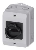
SENTRON, Switch disconnector 3LD, main switch, 3-pole, lu: 25 A, Operating power / at AC-23 A at 400 V: 9.5 kW, molded-plastic encapsulation for inch cable gland, rotary operating mechanism, black
