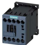
power contactor, AC-3e/AC-3, 7 A, 3 kW / 400 V, 3-pole, 480 V AC, 60 Hz, auxiliary contacts: 1 NO, screw terminal
