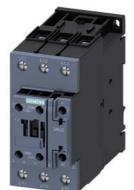
power contactor, AC-3e/AC-3, 51 A, 22 kW / 400 V, 3-pole, 24 V AC, 50 Hz, auxiliary contacts: 1 NO + 1 NC, screw terminal
