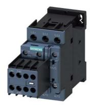
power contactor, AC-3e/AC-3, 9 A, 4 kW / 400 V, 3-pole, 24 V AC, 50 Hz, auxiliary contacts: 2 NO + 2 NC, screw terminal, removable auxiliary switch
