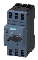
Circuit breaker size S00 for motor protection, CLASS 10 A-release 1.8...2.5 A N-release 33 A Spring-type terminal Standard switching capacity
