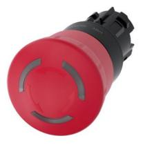
EMERGENCY STOP mushroom pushbutton, illuminable, 22 mm, round, plastic, red, 40 mm, positive latching, acc. to EN ISO 13850, rotate-to-unlatch
