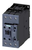
power contactor, AC-3e/AC-3, 51 A, 22 kW / 400 V, 3-pole, 110 V AC, 50/60 Hz, auxiliary contacts: 1 NO + 1 NC, screw terminal
