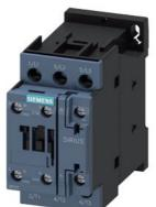
power contactor, AC-3e/AC-3, 32 A, 15 kW / 400 V, 3-pole, 220 V AC, 50/60 Hz, auxiliary contacts: 1 NO + 1 NC, screw terminal
