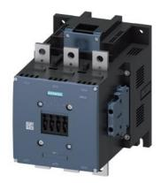
power contactor, AC-3e/AC-3 400 A, 200 kW / 400 V AC (50-60 Hz) / DC Uc: 380-420 V 3-pole, auxiliary contacts 2 NO + 2 NC drive: conventional main circuit: busbar control and auxiliary circuit: screw terminal
