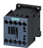
Coupling contactor relay, 3 NO + 1 NC, 24 V DC, 0.7 ... 1.25\* US, with integrated suppressor diode, Size S00, screw terminal suitable for PLC outputs
