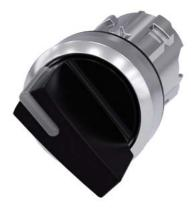
Illuminable selector switch, 22 mm, round, metal shiny, black, Selector switch short, 2 switch positions O<I, momentary contact type, Actuating angle  $45^\circ,\,10:30h/12h$
