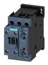
power contactor, AC-3e/AC-3, 12 A, 5.5 kW / 400 V, 3-pole, 24 V AC, 50/60 Hz, auxiliary contacts: 1 NO + 1 NC, screw terminal
