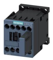
power contactor, AC-3e/AC-3, 12 A, 5.5 kW / 400 V, 3-pole, 24 V DC, 0.85-1.85\* Us, with varistor plugged on, auxiliary contacts: 1 NO, screw terminal, not expandable with auxiliary switch
