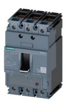
circuit breaker 3VA1 IEC frame 160 breaking capacity class H Icu=70kA @ 415V 3-pole, starter protection TM120M, AM, In=100A without overload protection short-circuit protection Ii=7...16 x In clamp connection
