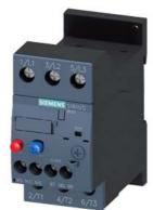
Overload relay 20...25 A Thermal For motor protection Size S0, Class 10 Stand-alone installation Main circuit: Screw Auxiliary circuit: Screw Manual-Automatic-Reset
