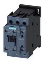
power contactor, AC-3e/AC-3, 25 A, 11 kW / 400 V, 3-pole, 220 V AC, 50/60 Hz, auxiliary contacts: 1 NO + 1 NC, screw terminal
