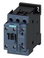
power contactor, AC-3e/AC-3, 32 A, 15 kW / 400 V, 3-pole, 110 V AC, 50 Hz, auxiliary contacts: 1 NO + 1 NC, screw terminal
