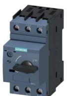
Circuit breaker size S00 for motor protection, CLASS 10 A-release 0.28...0.4 A N-release 5.2 A screw terminal Standard switching capacity
