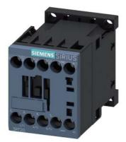
power contactor, AC-3e/AC-3, 12 A, 5.5 kW / 400 V, 3-pole, 110 V AC, 50 Hz / 120 V, 60 Hz, auxiliary contacts: 1 NO, screw terminal
